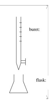
The flask contains a measured volume of the solution of unknown concentration, in this case 10.00mL of HCl<sub>(aq)</sub>, and the buret contains a standardized base, in this case 0.10M NaOH<sub>(aq)</sub>.
